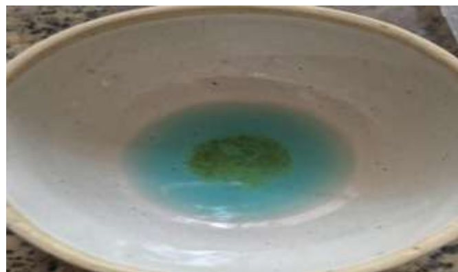
Figure 1. Colourimetric reaction between the Chen–Kao reagent and the standard mephedrone sample.
